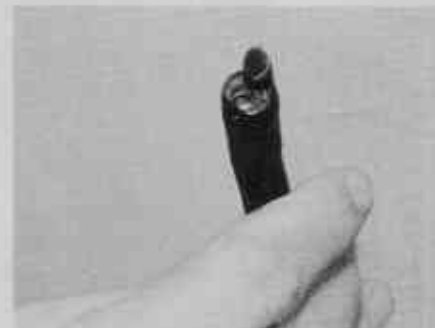
Tip of 1/2-inch-dia probe contains CCD TV camera and fiber optics for lighting.
