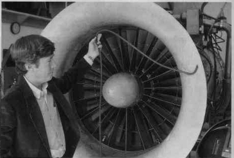
Ability of the probe to fly is demonstrated here; thrust of air jet holds end of probe suspended in position shown.
